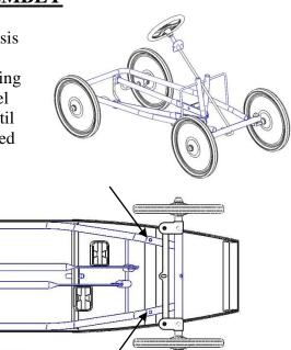
14. Drill (4)  $^{7}/_{32}$ " holes approx. as shown in chassis tube and crossmember and seat back and attach body with (4) provided machine screws.
