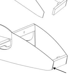
8. Fasten grill to right side as shown. Allow glue to set up before proceeding. 9. Attach crossmember in approx. location shown,  $\frac{3}{4}$ " above bottom of sides and 28.2" forward of the rear of the seat back.
