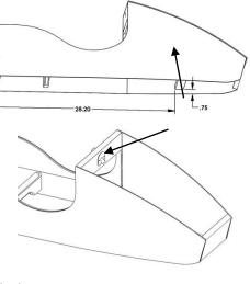
12. Glue front of hood to top of grill and allow to dry. (Be sure to apply glue to tops of sides before attaching hood to grill.)
